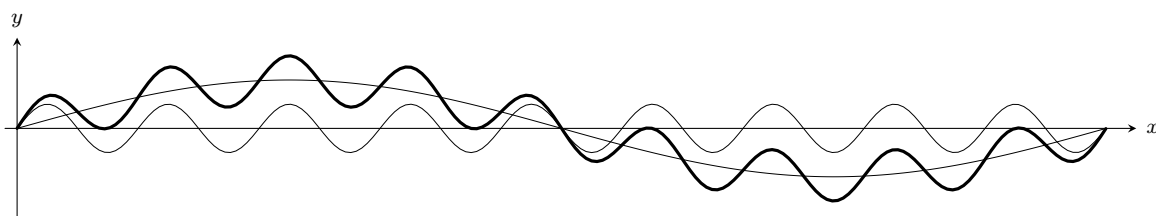
Figure 11: The addition (thick line) of two harmonic waves of widely different frequencies (thin lines).
