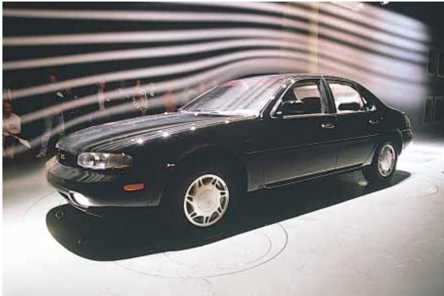
Figure 5: Laminar flow around an automobile in a test wind tunnel.
